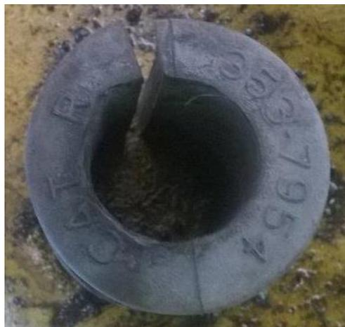
**Figure 3. These photos show wear to the corresponding surfaces of a hose and grommet that have been in service for 6500 hours. Accelerated wear occurs from the resulting clearance. In some instances, abrasive material can enter this clearance and further accelerate wear.**
