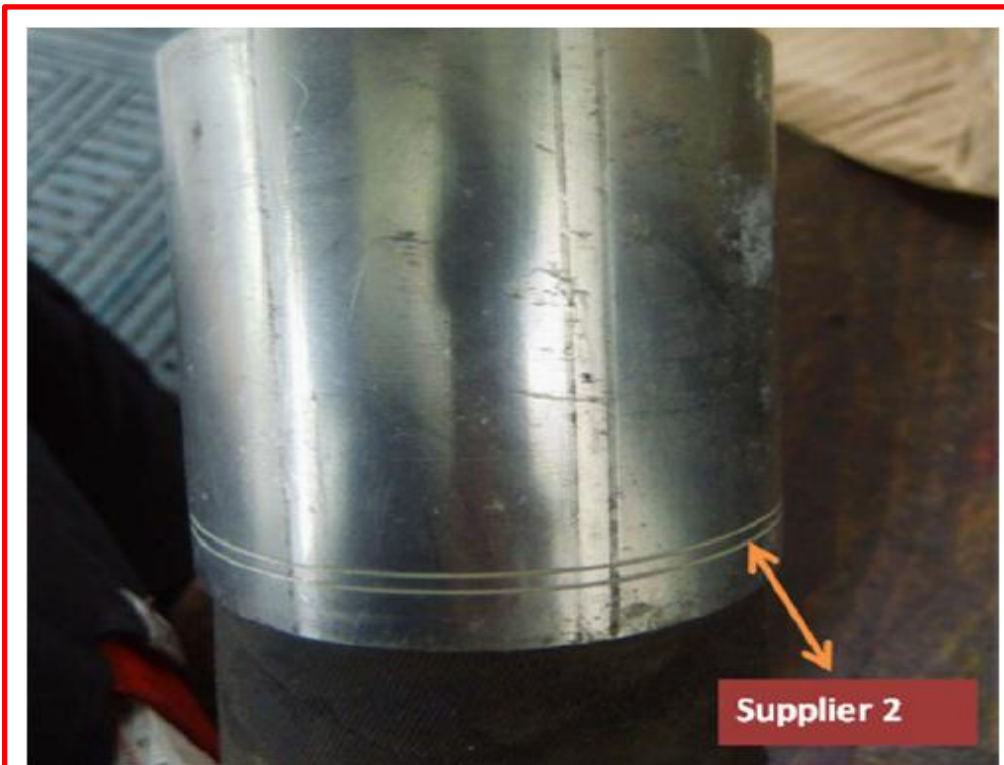
Illustration 4: Supplier 2 sleeve always with two machined rings on circumference. ( Bad )
