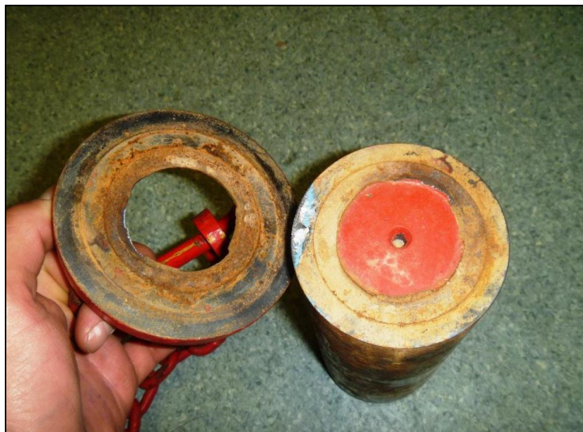
Figure 1 – showing lock pin failure mode
